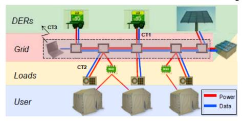
MIT study analyzed CT1 and CT2 and recommended MODBUS (industrial automation bus) to Ethernet TCP/IP. Also need to include:
